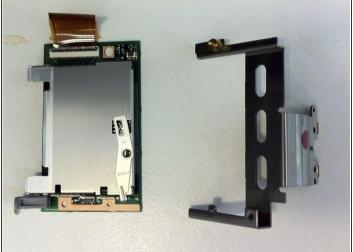
• Remove the two Phillips screws to separate the Holder from the Slot.
