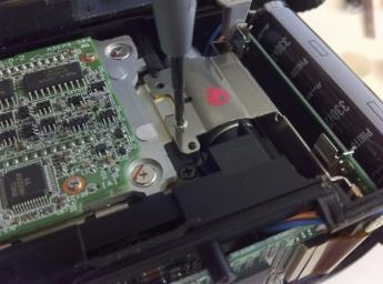
• Remove the two Phillips screws securing the holder of the CF Card Slot.
