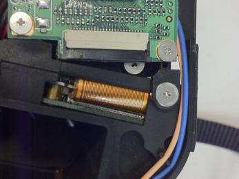
• Carefully fold the Pull the ribbon cable towards the CF Slot
