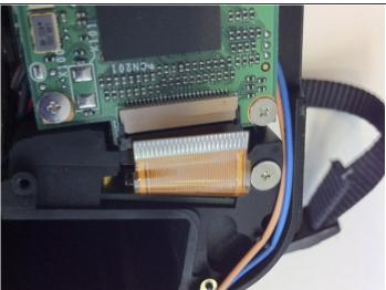
• Pull the ribbon cable out of its socket.
