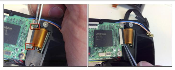
• Use Tweezers to open the locking on the ribbon cable socket.
