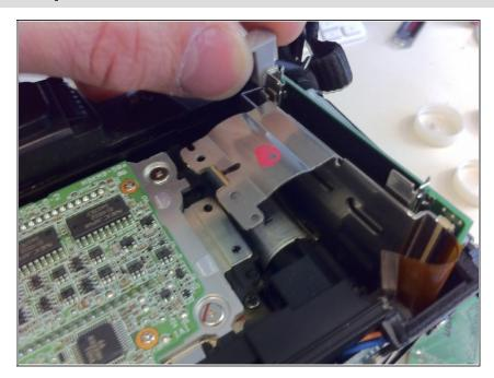
Pull the Slot out of the body.
