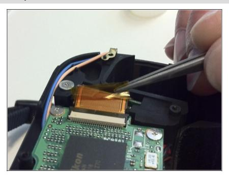
Peel of the Foil securing the Flexcable.
